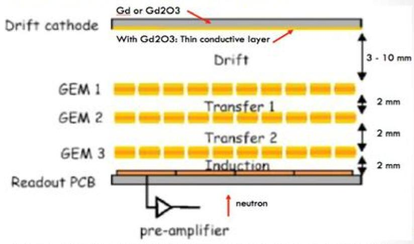
First measurements in backwards configuration with drift space of 3 mm and gain of 4000
