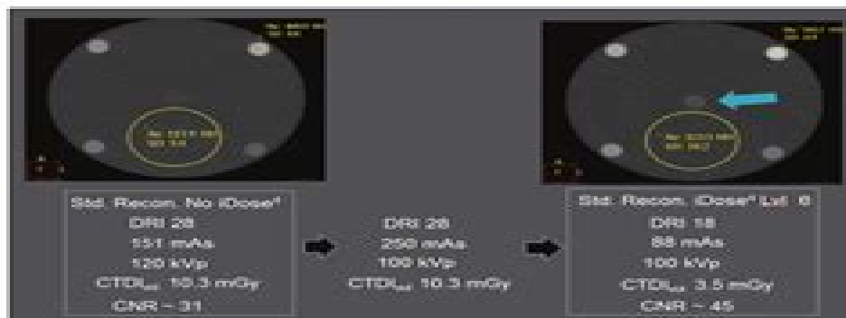
Figure 8 A 16 cm phantom with five iodine samples was used to show how the DRI can simplify adjustments in the tube potential, mAs, and iDose 4 . These adjustments lead to an increase in the CNR at low dose.
