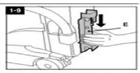
Slide rack down into place. Insert screw at (E) and tighten with a Phillips screwdriver.
