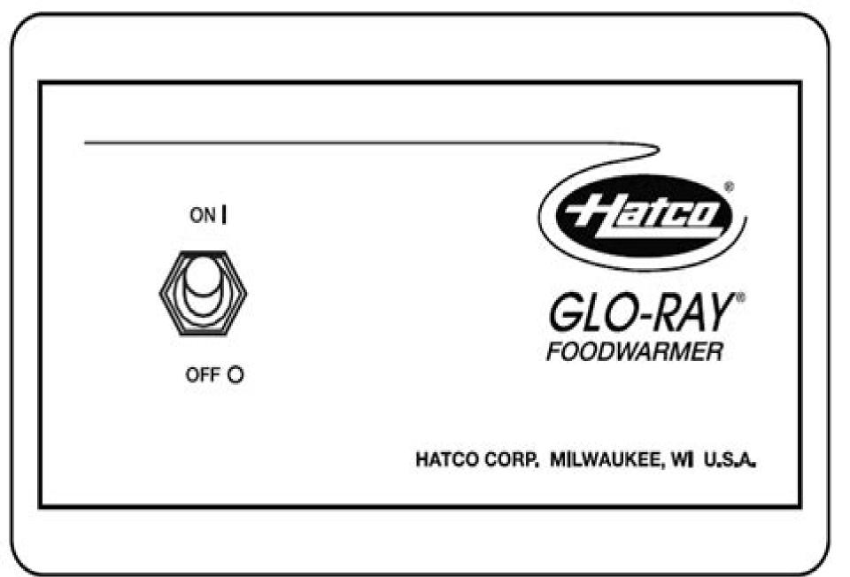
Control Panel with ON/OFF (I/O) Toggle Switch
