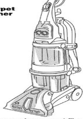
SteamVac™ All Terrain™ Cleaner cleans carpet fibers and hard floors by applying, scrubbing and removing hot tap water and cleaning solution.
