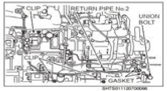
Replace old gaskets with new ones. Connect the return pipe No.2, and tighten a union bolt.
