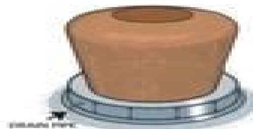
Figure 2-17: A mud-covered jute cloth jar mould. After about 30 minutes, the B. to become slightly dry before plastering the outside with cement mortar of 1:2 ratio.
