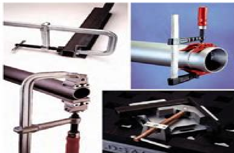
Figure 3-14. These various clamps are used to position and hold parts to be welded. (Bessey Tools North America)
