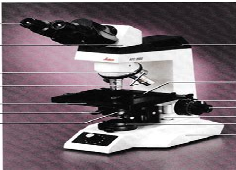
Figure 2.5 Compound light microscope.
