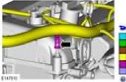
4. Disconnect the electrical connector and distact the was harriess retainers.
