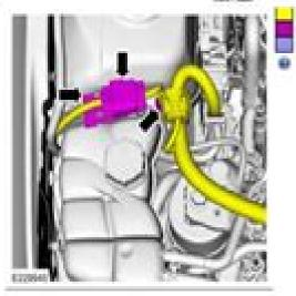
Remove the bolt and position the degas bottle sectio. Debuth the contact hope retainer.
