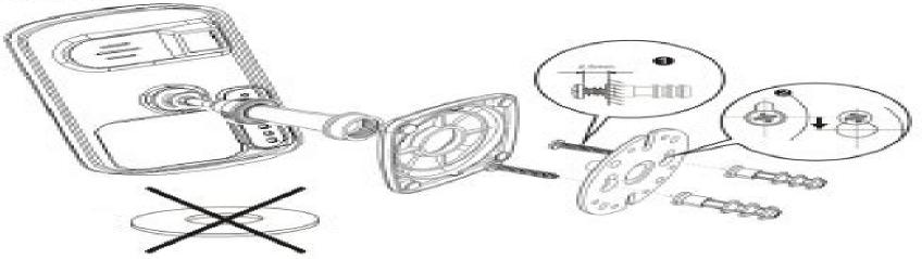
With the included screws and anchors, fasten the mounting bracket on to the wall. Then, reattached the base cover and screw the stand back on to the mounting bracket.
