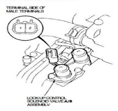
Measure the resistance between the No. 2 terminal solenoid valve A) of the lock-up control solenoid valve connector and body ground, and between the No. 1 terminal (solenoid valve B) and body ground.
