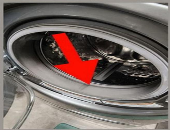
How To Remove Standing Water? Unclog Drain Holes On The Seal
