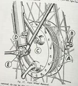
After removal, do not let the wheel fall on to the bush which projects from the broke storm side of the body pickenigh the both is pressed in, is may, if polyparted to a sharp blow, he farged back loco the hub. If this should happen, the bush can be recrimed and repositioned with the aid of the wheel spindle.
