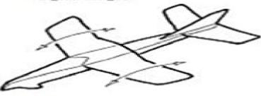
11 Add a bit of camber (front to back arching) to the wings, let it dry a bit, and you are ready for test flights.
