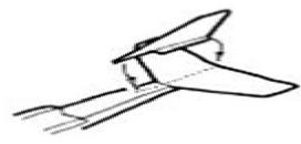
Ohie the rudder to the center of the stabilizer and the top of the fuselage. Take care to get it straight.
