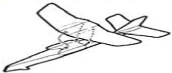
10 Glue the uring to the top of the finelage. The front edge is tucked and glued under the triangular tab at the back of part 10. The rear edge floats a bit at the back.
