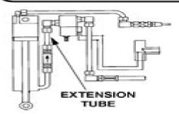
Remove the Coil Nut from the Lock Valve & Coil. Slide off the Coil and unscrew the Valve Cartridge (screwed into the Valve Block). Remove the bolts (if any), that secure the Valve Block to the Column.
