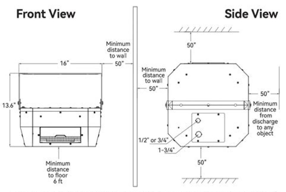
NOTE: Min. clearance to ceiling when not using mounting brackets is 1-5/8".
