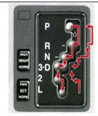
Shift while pressing the brake pedal. (Ignition switch must be in the "ON" position.)
