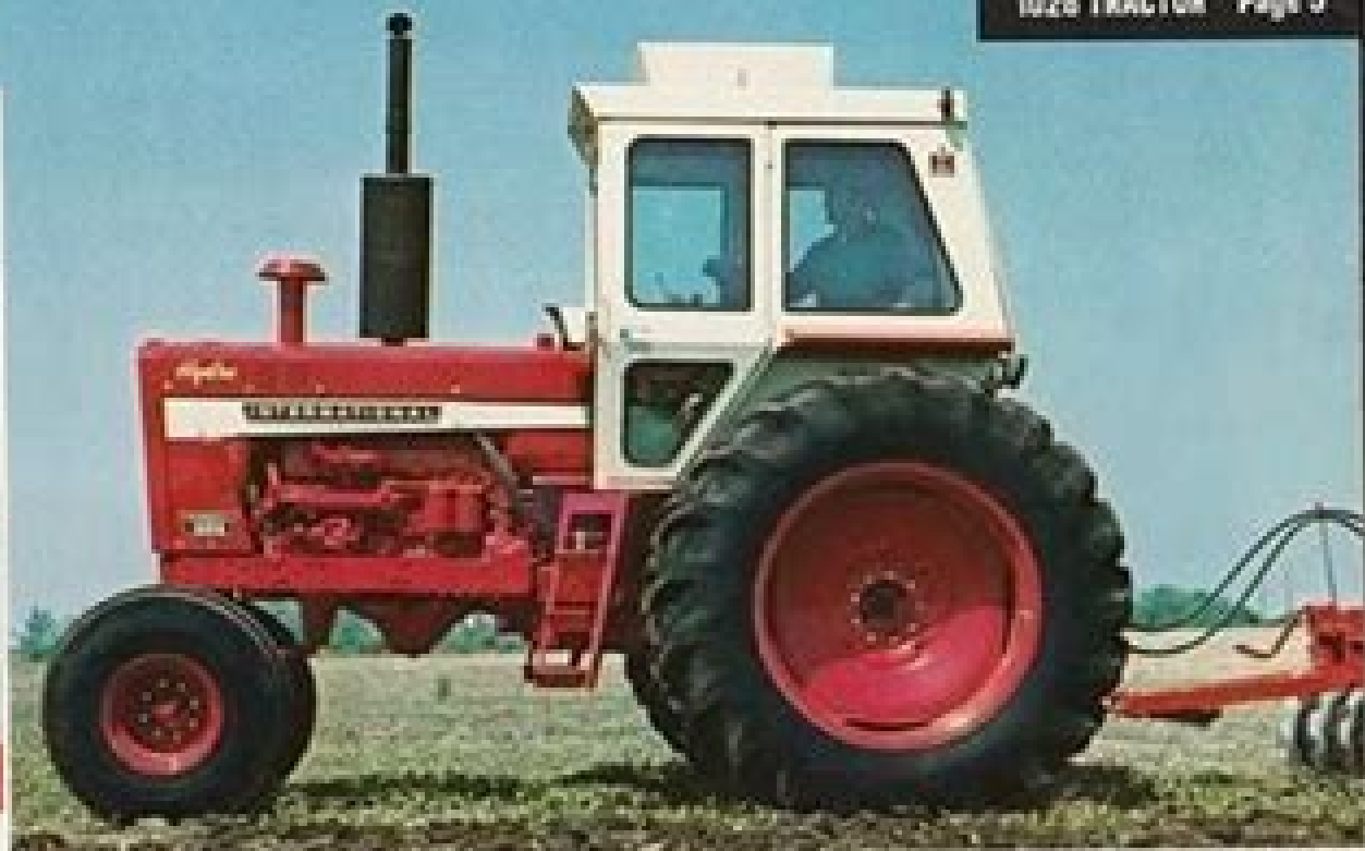
1026 HYDROSTATIC TURBO DIESEL 112.45 pto and 84.34 drawbar hp.
