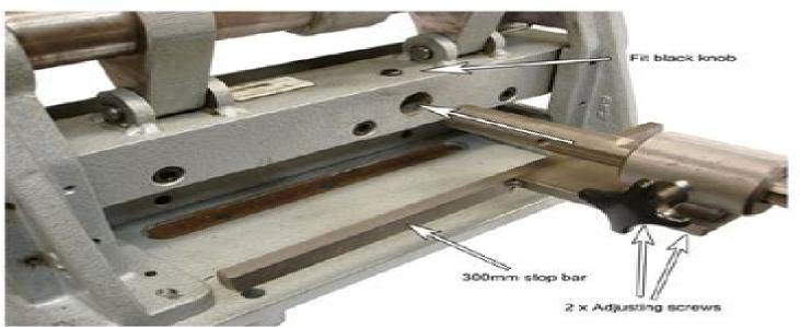
3. Fit the length stop bar to rear of machine by inserting the stop bar assembly into the 25mm diameter hole in top blade support block. Push the stop (300mm bar) against the top blade. (This bar can be adjusted by undoing the two screws underneath). Align the edge of the knurled circular block with the zero on the scale which is attached to the 25mm diameter bar and tighten the black knob on to the assembly.
