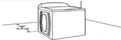
Move washer to within 4 ft. (1.2 m) of its final location; it must be in a fully upright position.
