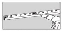
Fasten your rails, base rail first. Make sure you've found suitable points in the wall where the rails can be fastened and that the rails are level before drilling.
