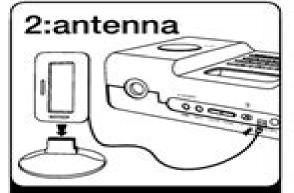
Snap AM antenna into provided stand, then plug antenna cable into socket on back of iH8. Move antenna 12" away.
