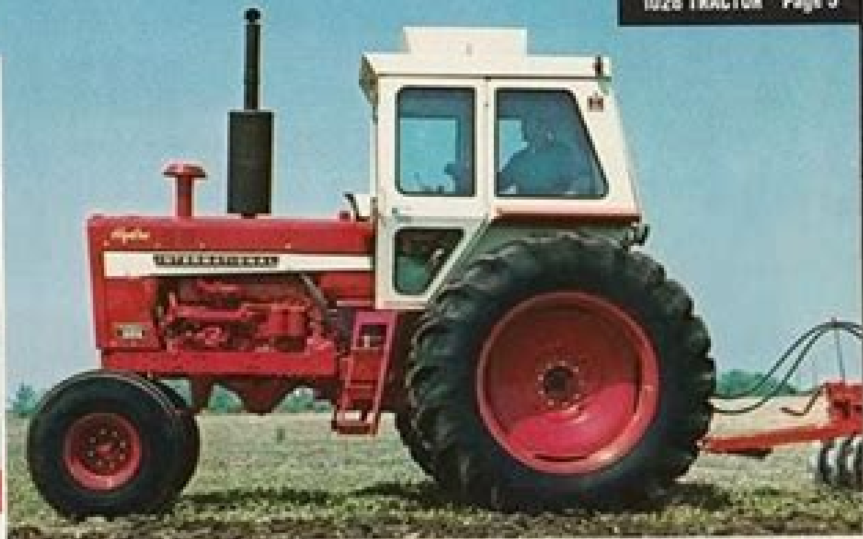
1026 HYDROSTATIC TURBO DIESEL 112.45 pto and 84.34 drawbar hp.
