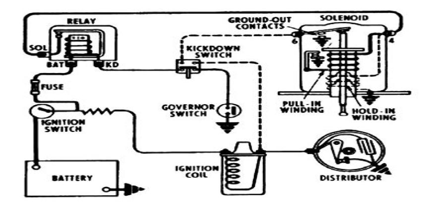
Overdrive Electrical Circuit Wiring Diagram
