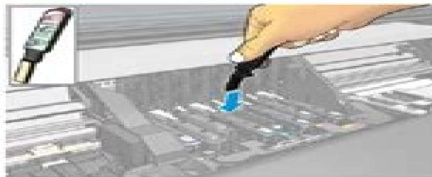
7. Rub the sponge against the contacts with a light force along the entire depth of the flex connector, inserting the wiper as far as allowed by the mechanical stop on the tool.
