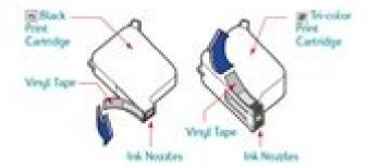
5 For each print cartridge, lift the cradle latch inside the printer. With the copper electrical contacts toward the rear of the printer and the print cartridge held vertically, push the print cartridge firmly down into the appropriate cradle.
