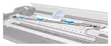
16. Leave the flex retainer with the trailing cable in the position shown below.
