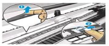
15. Slide the flex retainer with the trailing cable to the right. Be careful not to damage the trailing cable.
