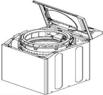
7. Remove Inner Tub Bolts and Inner Tub.
