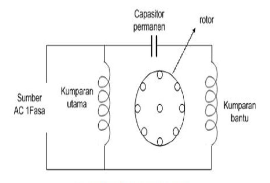
Gambar 04, Motor running kapasitor
