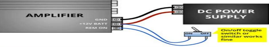
If you're using a line level converter, you can optionally use one with a remote wire output built in. The amp will turn on and off automatically with the speaker level input signal. These types need power to be connected also.
