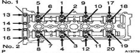
Install and uniformly tighten the 20 bearing cap bolts in several passes, in the sequence shown. Torque:
