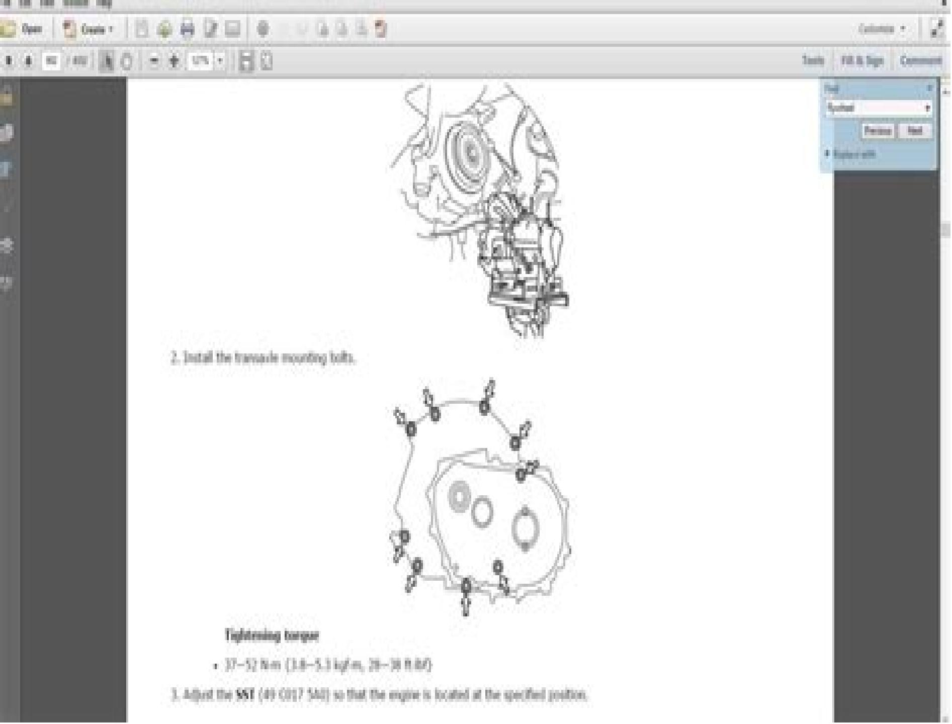
2. Install the transverse mounting bolts.
