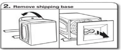
To avoid damaging floor, place cardboard supports from shipping carton on floor behind washer. Tip washer back and place on cardboard supports. Remove shipping base. Set washer upright.
