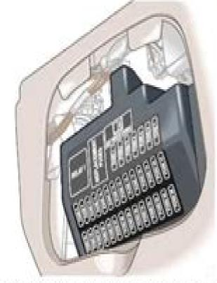
The passenger compartment fuse box is located on the right-hand side trim panel in the footwell. Remove the fuse box lid by pressing the retaining lugs and lifting.
