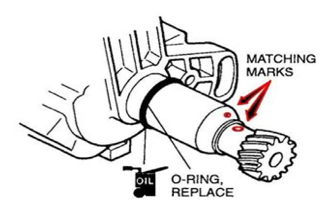
Fig. 1: Camshaft/Distributor Matching Marks
