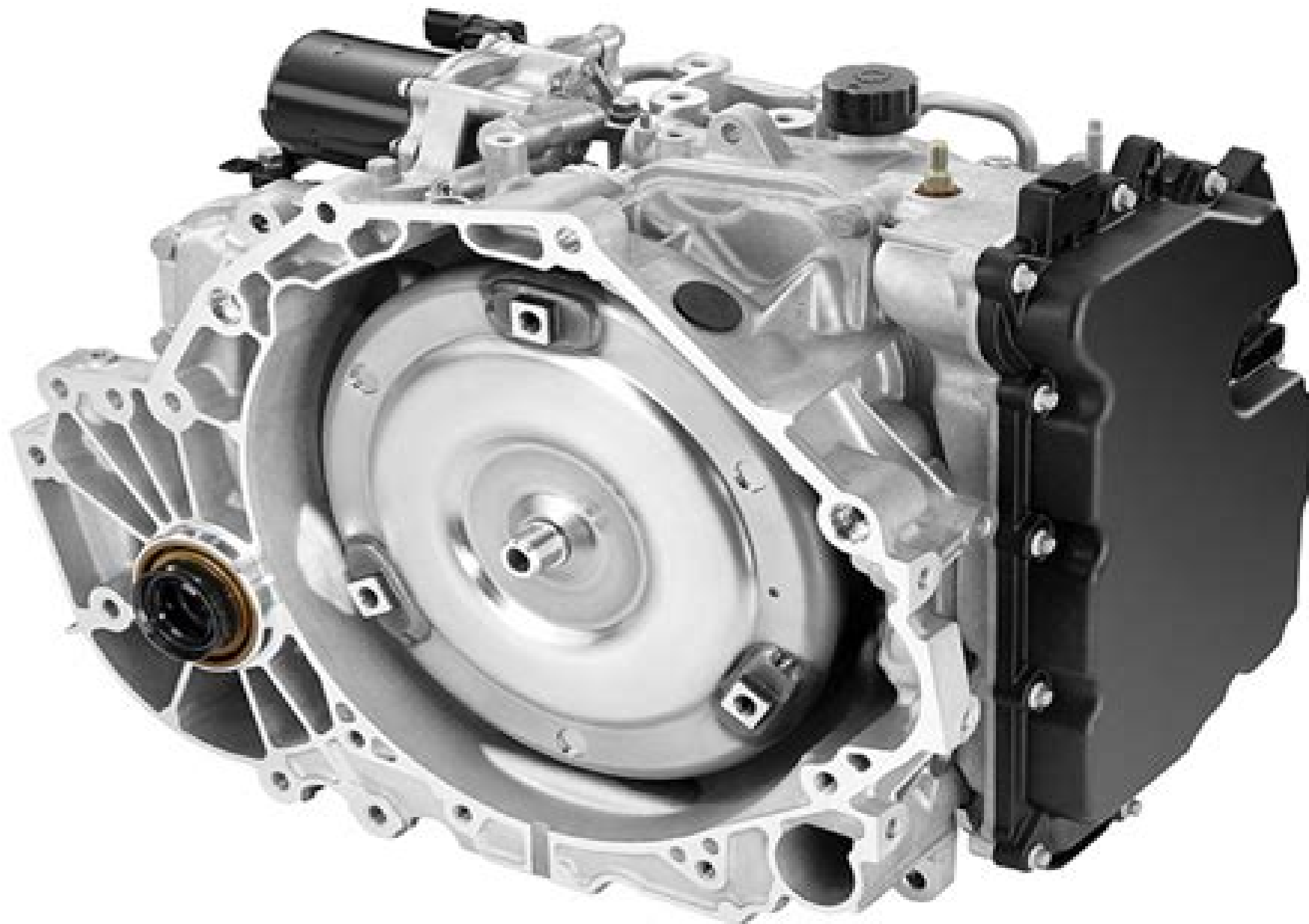
2014 Hydra-Matic 6T40 (MNI) Six Speed FWD Automatic Transaxle with Auxiliary Pump for eAssist
