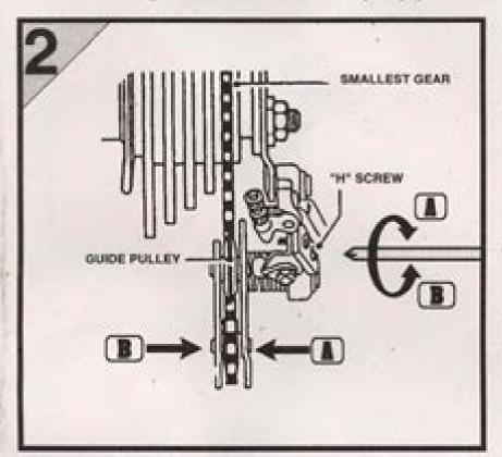
Use the "H" screw to adjust so that the guide pulley moves to directly below the smallest gear.
