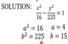
The narrowest part of the cooling tower is 2a. So, it measures 8 meters.
