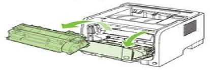
Remove the new print cartridge from the bag. Place the used print cartridge in the bag for recycling.
