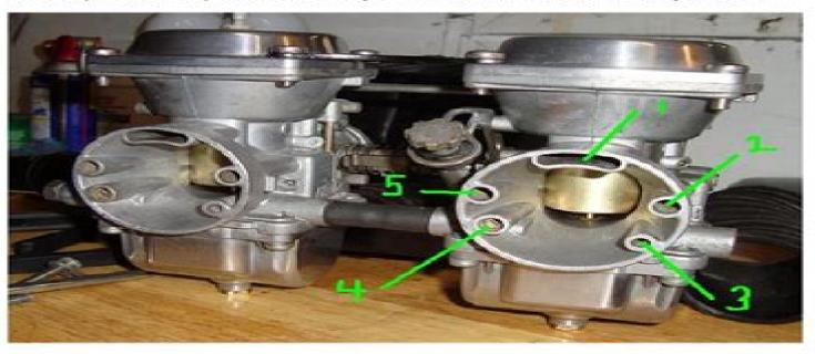
May visualize from this BS34 diagram how turning the pilot screw in clockwise reduces the volume of mixture through the orifice into the carb bore (which produces a leaner mixture into the combustion chamber), and how turning the pilot screw out counter-clockwise increases the volume of mixture through the orifice into the carb bore (which produces a richer mixture into the combustion chamber).
