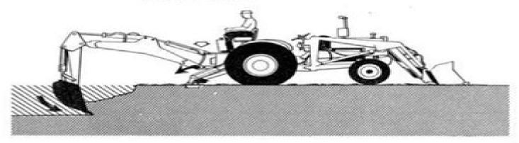
Counterweighting is particularly critical when operating the backhoe in the extreme awing positions, because the tendency in to lift one stabilizes and transfer the total weight of the unit to the other stabilizes.
