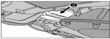
The frame serial number ① is stamped on the right side of frame under the footboard.
