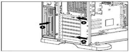
11. Turn the spring-loaded locking pin until it locks into the chassis.
