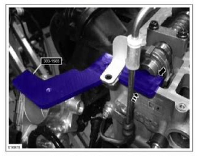
NOTE: The crankshaft must remain in the <u>TDC</u> position during removal of the pulley bolt or damage to the engine can occur. Therefore, the
