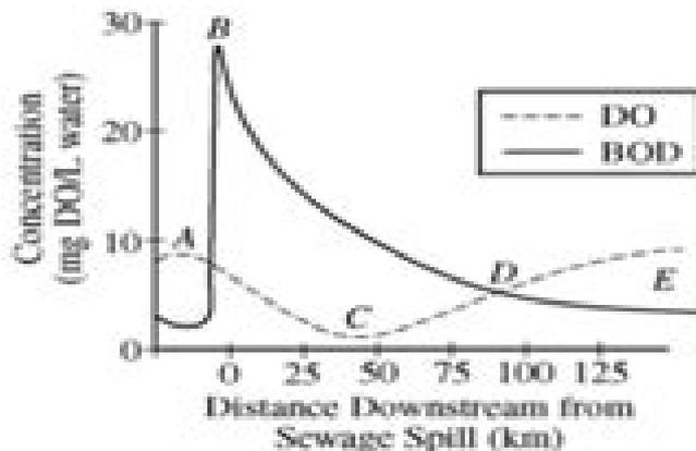
19. The graph above shows the effect of sewage on biological oxygen demand (BOD) and dissolved oxygen (DO) in a flowing stream. The smallest fish populations will most probably be found at point
