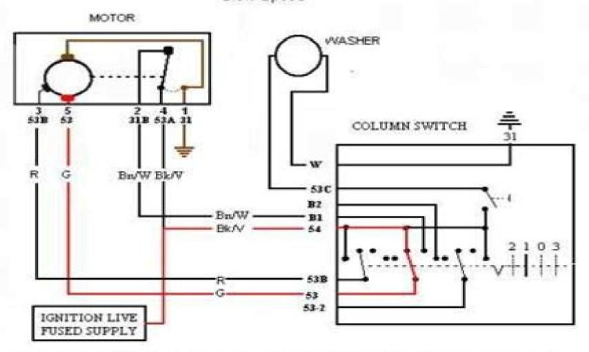
With the column switch set to slow speed and the ignition on, there is a fused ignition live supply to contact 54 on the switch. This is connected internally through the switch to feed current out through 53 on the switch which is wired to 53(5) on the motor and current thus flows through the slow speed circuit, driving the motor, and out to earth via motor contact 31(1).
