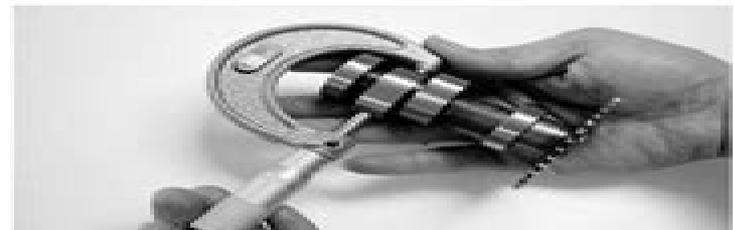
Check each camshaft bearing for play or damage. Replace the camshaft assembly with a new one if the bearings are noisy or have excessive play.
