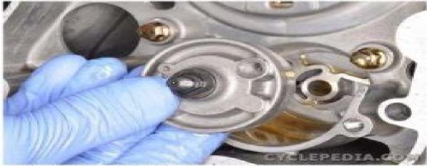
Remove the oil pump from the engine. Turn the oil pump shaft and make sure it turns smoothly.
