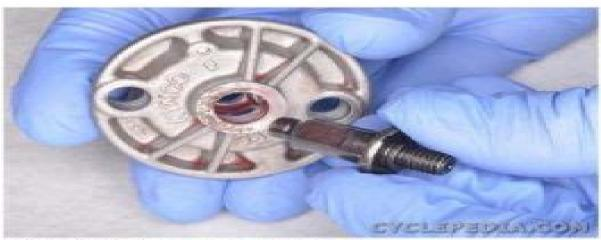
Slide the oil pump shaft out of the oil pump.
