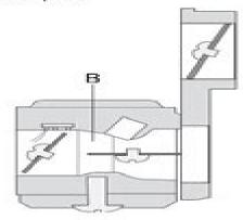
In the pump unit (C), fuel is pumped from the fuel tank to the metering unit. One side of the pump diaphragm is connected to the crankcase and pulses in time with the pressure changes in the crankcase. The other side of the diaphragm pumps the fuel.
