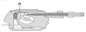
The mixing venturi (B) houses the choke, throttle valve and diffuser jets. Here air is mixed with the fuel to give a fuel/air mixture that can be ignited by the ignition spark.
